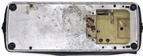
These two views of the underside of the show the battery compartment and the chassis base-plate together with the recessed 2-pin socket for the 240VAC mains input. The cover for the socket is missing.
