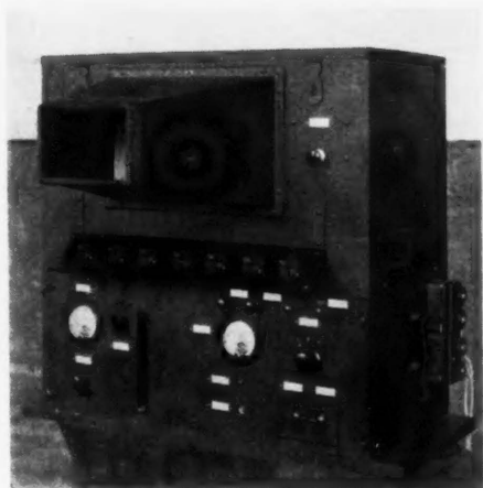
Production testing apparatus developed in 1931 for visual indication of faulty components
