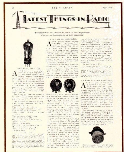
IN 1929 THE 4-ELECTRODE screen-grid UY-224 and a 0.125-watt potentiometer were the latest developments in radio.
