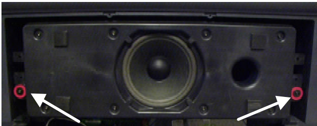
Screws Securing Subwoofer
