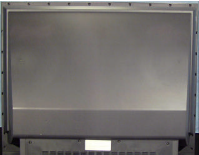
20 Screws Secure Protective Screen Frame
