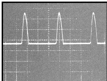
59 29V_{p-p} 10V/20\mu sec/div.
