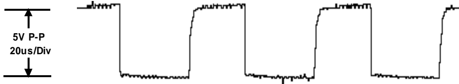
Figure 18, Horizontal Drive U1001 Pin 23
