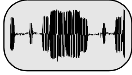
③ 5.36V p-p IC3001 PIN 34 C_IN
