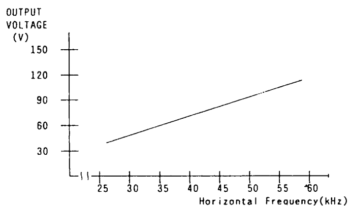
(Fig 1-2-6) Relationship of the Horizontal frequency and the F B T's DC Supply Voltage
