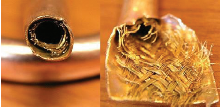
Figure 4. Screen mesh wick [15].
