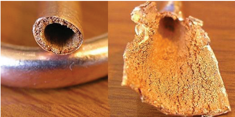
Figure 2. Metal sintered powder wick [15].
