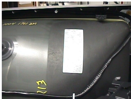
Fig. 2 Mount the X-ray CRT label on the CRT bell.
