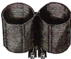
The "Lekeless" Transformer Tuned Radio Frequency
