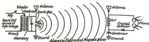
SENDING AND RECEIVING (damped waves) This sending arrangement causes interference and cannot be used by amateurs.
