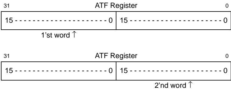
Figure 4-5-7 Register Operation for DMA Access in 16-Bit Width (ATF)
