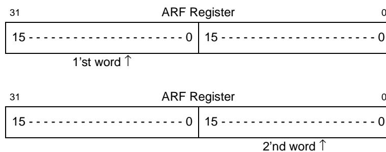
Figure 4-5-8 Register Operation for DMA Access in 16-Bit Width (ARF)
